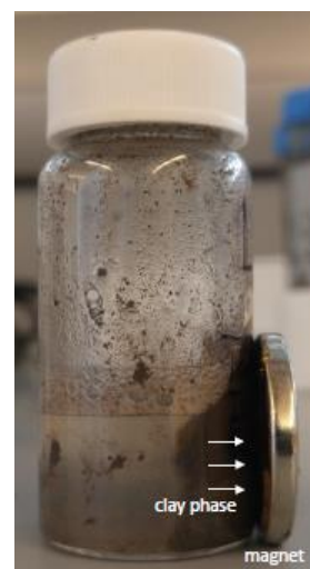
Figure 2: MFT treated with IL that had been premixed with superparamagnetic iron oxide nanoparticles. Clay has been magnetized and can be attracted to the side of the vessel using a magnet.
